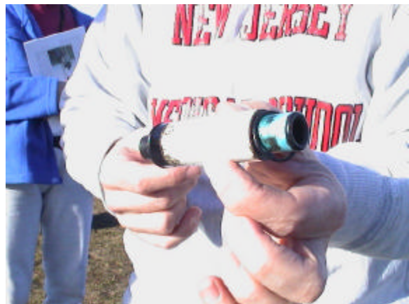
Reload removed intact from its casing, demonstrating the “anatomy” of an RMS motor.
