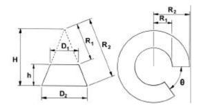
A transition has an upper diameter  $D_1$ , a lower diameter  $D_2$  and a height h. The first task is to find H, the height of the cone from which the transition has been taken. Now, anywhere along the cone, the ratio of the height from the tip, to the diameter, will be the same. So:
