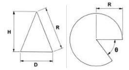
A cone of base diameter D and height H can be made from a circle of radius R, with a wedge of angle  $\theta$  cut from it. R is also the distance from the tip of the cone to the edge of the base, and is given by:
